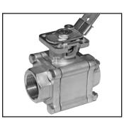
TRIAD SERIES 66FD-62011 API 607 4TH EDITION FIRE RATED SIZE: 1/4" - 4" NPT, SW AND BW 2000 PSI 1/4" TO 1" 1500 PSI 1-1/4" TO 2" 1000 PSI 2-1/2" TO 4" STAINLESS STEEL ISO 5211 DIRECT MOUNTING PAD LOCKING DEVICE OPTIONAL V BALL
