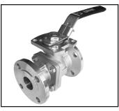
TRIAD SERIES 9150/9300/9600 API 607 4TH EDITION FIRE RATED SIZE: 1/2" - 12" ANSI 150#, 300# & 600# FLANGED STAINLESS STEEL / CARBON STEEL ISO 5211 DIRECT MOUNTING PAD LOCKING DEVICE OPTIONAL V BALL \*METAL SEATING AVAILABLE
