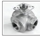
**TRIAD SERIES 33D** SIZE: 1/4" - 2" 1000 PSI 1/4" TO 1" 800 PSI 1-1/4" TO 2" STAINLESS STEEL TWO PIECE THREE WAY L PORT OR T PORT ISO 5211 DIRECT MOUNTING PAD \*AVAILABLE IN BRASS SIZE: 1/4" - 3"
