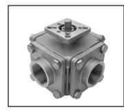
**TRIAD SERIES 36 AND 46** SIZE: ½" - 10" THREE WAY & FOUR WAY FOUR SEATED NPT, SW, BW, 150# & 300# FLANGED 1000 PSI 1/4" TO 1" 800 PSI 1-1/4" TO 2" L PORT, T PORT OR X PORT STAINLESS STEEL / CARBON STEEL ISO 5211 DIRECT MOUNTING PAD LOCKING DEVICE
