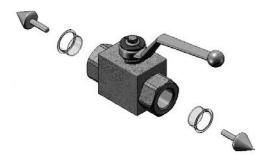
• When tightening onto the pipe, never hold the valve by the open/close lever, but use a wrench on the hexagon plug.
