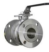
8.8 Cycle the valve slowly, with a gentle back and forth motion, to build gradually to the full quarter turn. By cycling slowly, the seat lips will assume a permanent seal shape against the ball. A fast turning motion, at this point, may cut the seats before they have a chance to form the proper seal.
