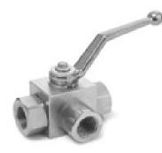
• The XHP3W three way value is typically supplied with an L Port ball configuration. The most common use of the value is to direct flow into the center port and by turning the handle 90° flow can be diverted to either side outlet port. The illustration below depicts the handle position as it relates to the flow path.
