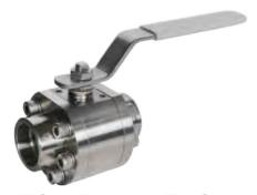
Series B1000 3 PIECE, Full Port Threaded / Socket / Butt Weld End PRESSURE: 1000 psi SIZE: 1/4" ~ 2"
