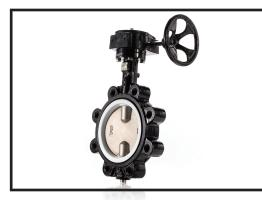
TRIAD SERIES 750 / 751 SIZE: 2" - 40" LUG OR WAFER DEAD END SERVICE LUG STYLE 200 PSI EPOXY COATED DUCTILE IRON BODY 316 SS DISC EPDM, BUNA N, VITON OR PTFE LINERS ISO 5211 DIRECT MOUNTING PAD
