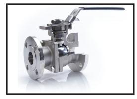
**TRIAD METAL SEATED VALVES** SEATS: ALLOW 6 / STELLITE BALL: ENP OR HARD CHROME PLATED TEMPERATURES: TO 1200° F
