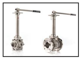
TRIAD CRYOGENIC VALVE SERIES 60C/70C/80C/90C/93C SIZE: 1/2" - 4" NPT, SW, BW ANSI 150# & 300# FLANGED STAINLESS STEEL SEATS: KEL-F (PCTFE) TEMPERATURE: -321° TO 392° F ISO 5211 DIRECT MOUNTING PAD LOCKING DEVICE OPTIONAL V BALL
