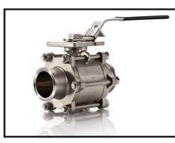
TRIAD SERIES 920-62011 SIZE: 1/2" - 4" 1000 PSI CLAMP END VALVE STAINLESS STEEL CAVITY FILLED THROUGH PORT DESIGN ISO 5211 MOUNTING PAD LOCKING DEVICE \*MODEL 920D DIRECT MOUNT ALSO AVAILABLE
